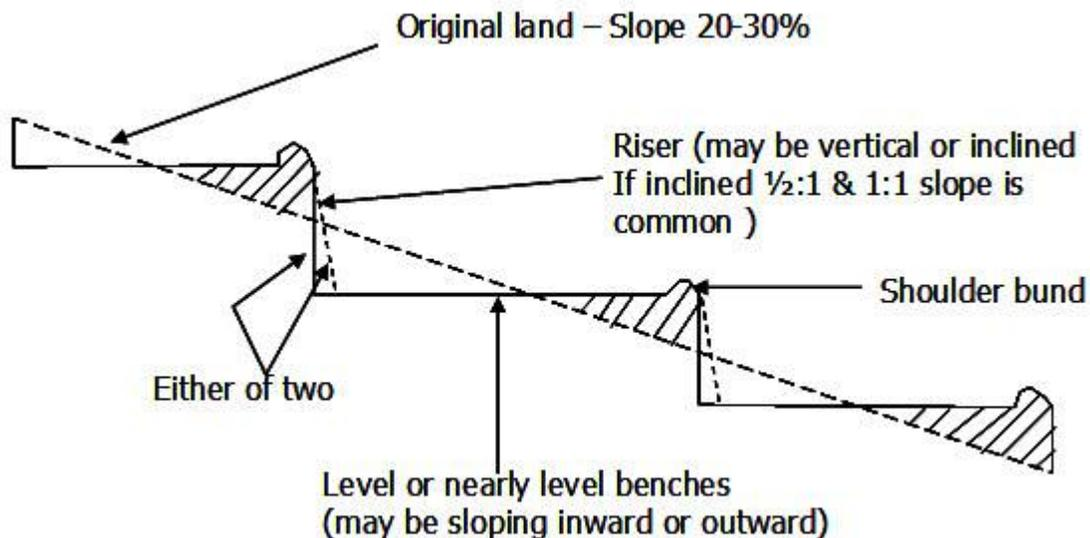
**Fig. 5.2. Bench terrace and its different components.**
