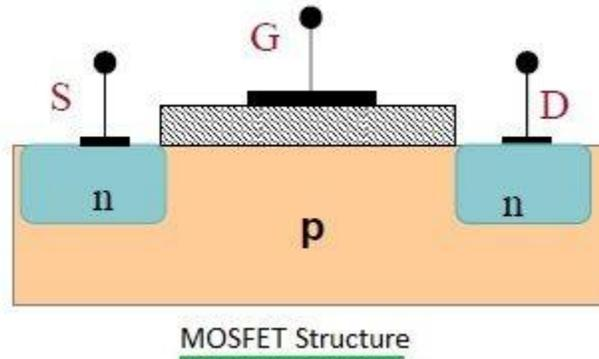
The working of a MOSFET depends upon the MOS capacitor. The MOS capacitor is the main part of MOSFET. The semiconductor surface at the below oxide layer which is located between source and drain terminals. It can be inverted from p-type to n-type by applying positive or negative gate voltages.
